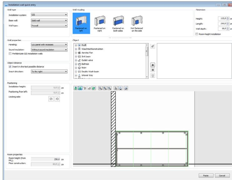
The quick entry window includes different areas, such as Wall type and Wall coupling, which you can use to plan an installation wall in steps. The choice of a wall type affects the visualisation of the wall coupling and the input options for the dimensions. Therefore always adhere to the following principle when planning: **from left to right and from top to bottom**. This procedure will become clear in the following example.
