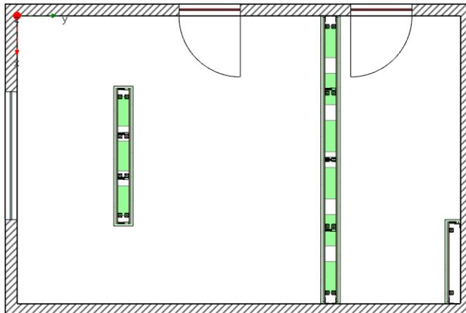
**Inserting a part-height prewall**
