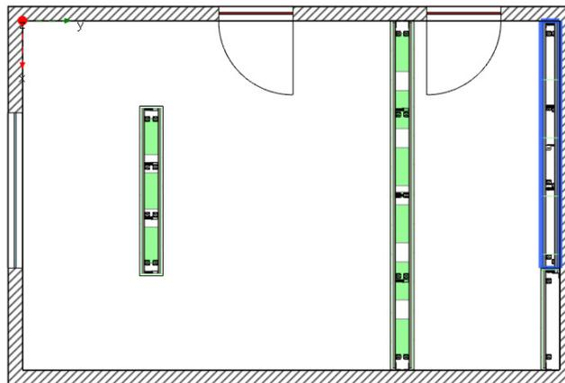
**Inserting the second room-height prewall**
